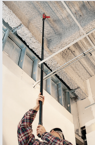
Ramset Pole Tools are an excellent choice for high-reach fastening applications.
